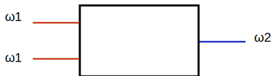
(a) Draw of the second harmonic generation in a non linear crystal
